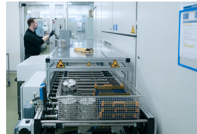
The new intermediate production cleaning system significantly reduces the amount of waste water.
