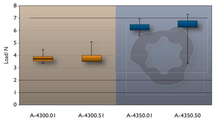
Figure 9: Results of fatigue testing of conventional (yellow background) and TriLock plates (blue background); Left fatigue life, right: fatigue strength. Fatigue strength is significantly higher for the TriLock plates, fatigue life can not be compared directly due to the differing load profiles (Figure 6).
