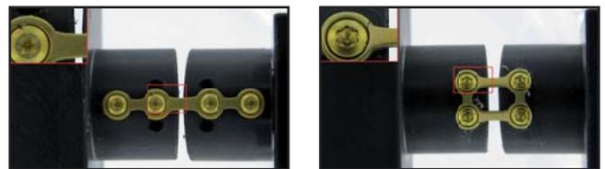
Figure 8 Non-locking plates after testing. Left: A-4300.01 (buckled), right: 4300.51 (fractured)
