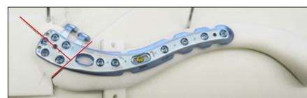
Fig. 2: Superior lateral plate setup, fracture line shown in red
