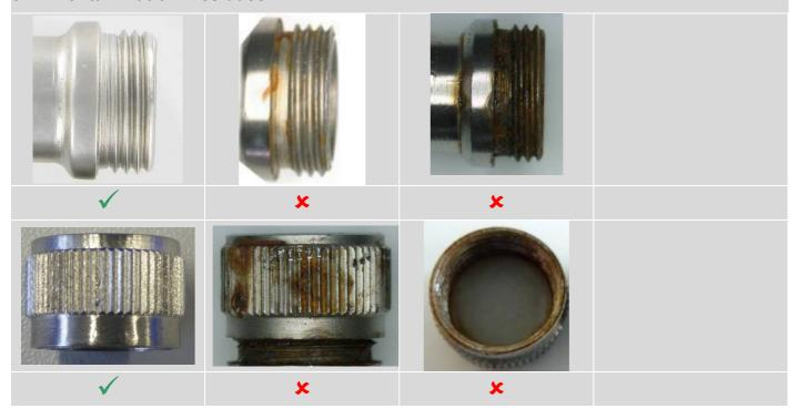
**Possible damage** K-wire dispenser is contaminated with:
